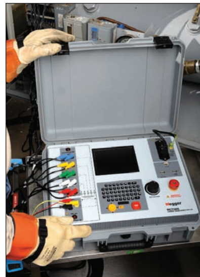
With a manual voltage output control knob, the user is able to perform any test required manually if only a spot check is required.
